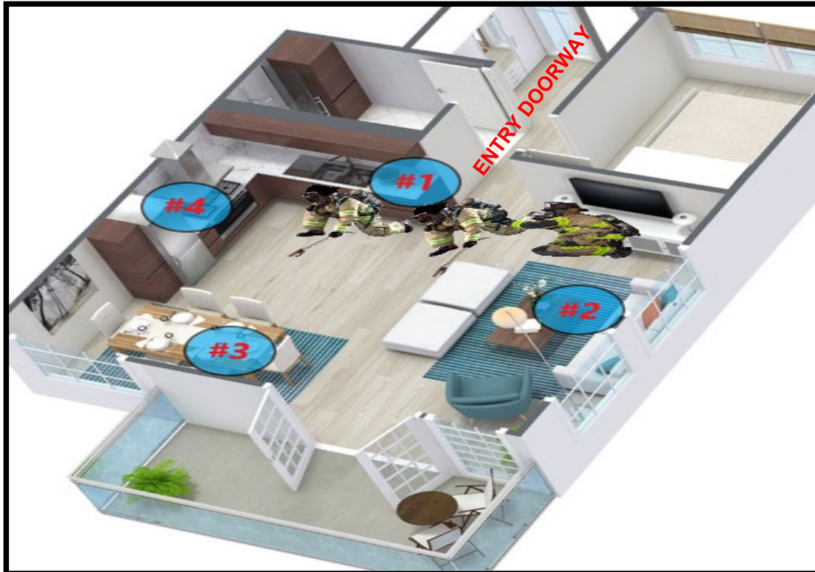
(FIGURE 1) WALL NUMBERING. '1' WALL IS THE ENTRY WALL THAT CONTAINS THE DOORWAY THE SEARCHERS CURRENTLY OCCUPY. THE '2', '3', AND '4' WALLS GO CLOCKWISE AROUND THE SPACE.
